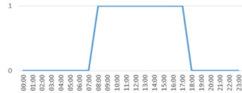
Figure 6: Heating and Cooling schedule.
